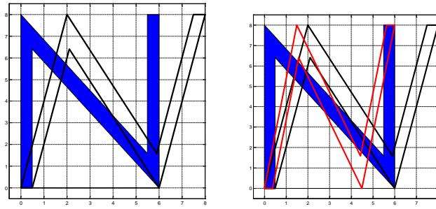
7.18  $\begin{pmatrix} -2.464 \\ 3.732 \\ 0 \end{pmatrix}$ . The transformation resulted in robotic arm rotating  $60^\circ$  in  $(x,y)$  plane.
