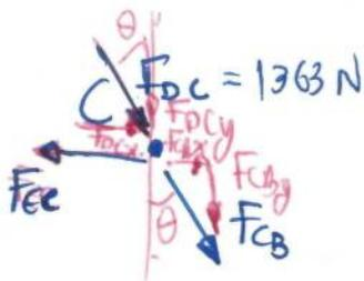
The direction of force F<sub>DC</sub> is known because it was found when applying the condition of equilibrium at point D.
